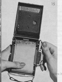
tective paper, so that its beginning can be inserted into the wider slot of the take-up spool. Tighten the protective paper by turning the folding film winding key (22) several times. Take care that the protective paper remains smooth on both sides of the spool when being wound on Close the camera back. Turn the film winding key (22) until number "1" appears in the film window. After the film window has been closed the SUPER IKONTA is ready for the first exposure.
