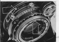
everything from 14 ft. to infinity will be recorded sharply. According to the prevailing lighting conditions exposure times of <sup>1</sup>/<sub>25</sub>, <sup>1</sup>/<sub>50</sub> or <sup>1</sup>/<sub>100</sub> sec. have to be
