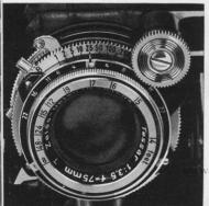
You can, of course, also proceed the other way round, i. e. measure the front and the rear limit of the area that has to be reproduced sharply and then determine the required lens stop by means of the depth-of-focus scale.
